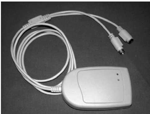
Fig. (3). RFID tag Reader to be connected to a computer in the keyboard jack.
