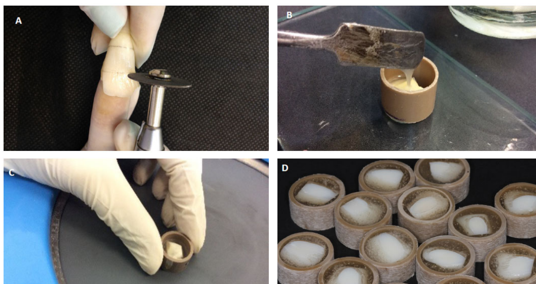
Fig. (1). (A) Standardized measurements of the middle third for making the specimens; (B) tooth fragment adapted with the buccal side down being included with autopolymerizable resin; (C) specimens being polished after 24 hours of embedding and (D) finished specimens.
