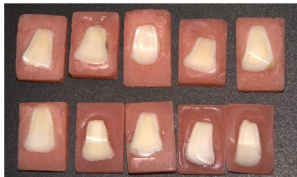
Fig. (1). Mounting of the tooth samples in the acrylic resin and exposing the buccal dentin.
