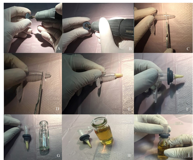
Fig. (2). Microleakage was assessed by using a two-chamber model. A, B: A hole was created in the rubber stopper of the penicillin bottle by using an acrylic bur. C, D: The microtubes were cut-ended. E: The prepared root (cut at the cemento-enamel junction) was placed in cut-end microtubes such that the coronal 2 mm of the tooth was inside the microtube and its root was out of it. F, G: The tooth/tube was then inserted through the created holes. H: Sterile Brain Heart Infusion (BHI) broth was added to the vials until it covered the apical 2 mm of each root. I: The tooth/microtube interface and the microtube/cap interface were sealed with glue.
