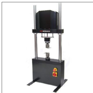
Fig. (2). Universal mechanical testing machine for measuring load on teeth assessing resistance to fracture.
