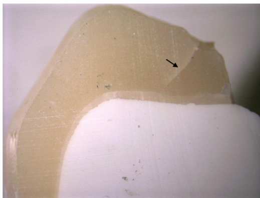
Fig. (3). Microscopic image (2.5x magnification) showing cone crack (arrow) starting at the loading area which propagates till cement layer.
