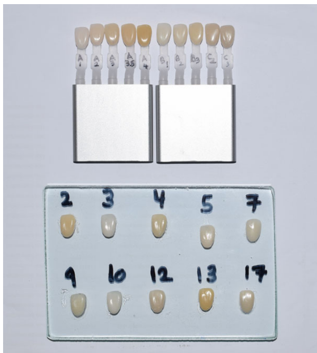
Fig (1). A glass-slab with 10 cured composite samples randomly numbered, and a custom shade guides made from the same composite material (ZENIT Nano, President Dental, Germany).
