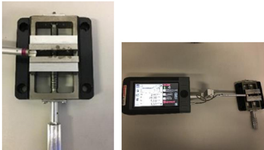
Fig. (3). The specimen was placed on the flat table surface, and a clamp was used to hold specimens stable in its position (A), the values of surface roughness were displayed digitally on the screen of the portable digital roughness (SR 300, Taylor Hobson, Leicester, England) (B).
