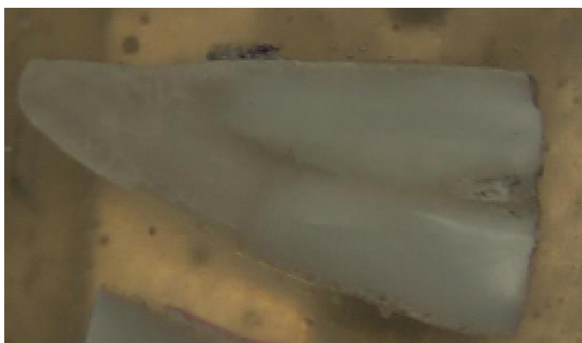
Fig. (1). Root section was embedded in self-curing acrylic resin, and the root canal dentin surface was facing up.
