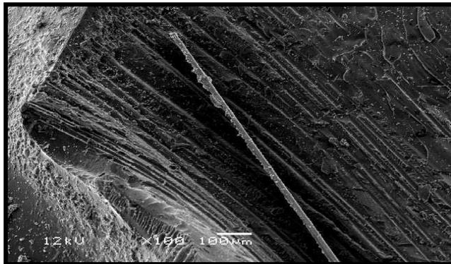
**Fig (8).** Cohesive failure with Scotchbond as observed under SEM at x100 magnification. Note the glass fibers.
