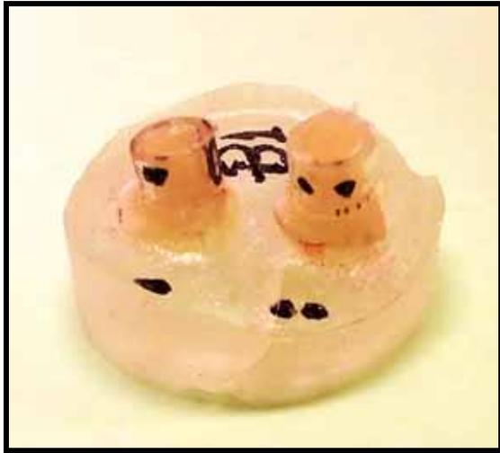
**Fig (1).** The cylinders filled with composite material attached to the glass-fibers ribbon bonded to primary molars enamel surface after embedding.
