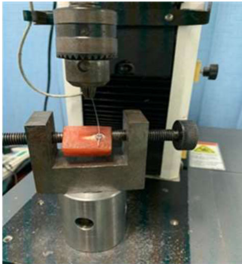
Fig. (4). Test setup with acrylic block model in instron universal testing machine.
