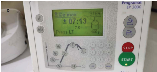
Fig. (4D). Setting up the thermal injection device.
