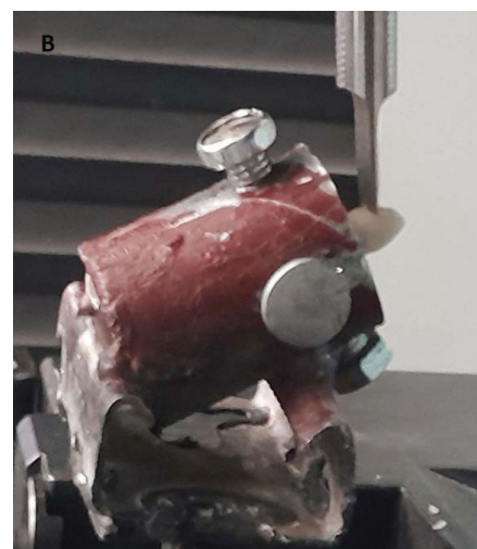
Fig. (8B). Applying oblique forces to the teeth at a 45-degree angle on a custom-made base.
