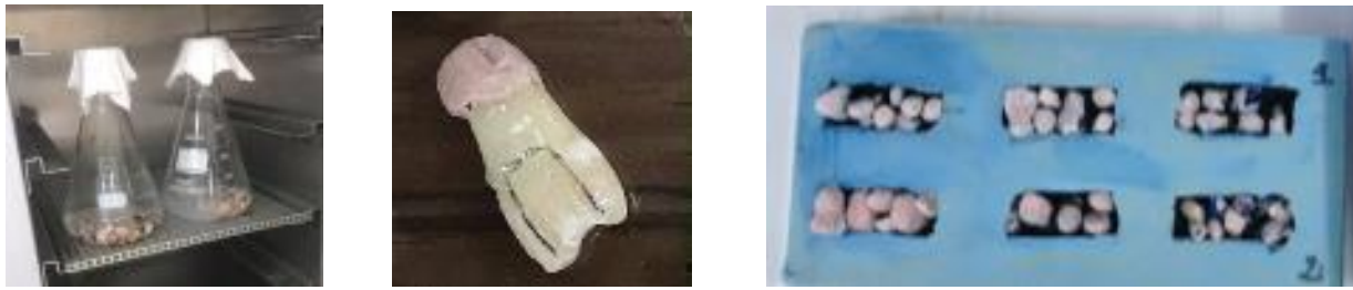
Fig. (4). Thermocycling,application of two coats and immersion of teeth in methylene blue. After removing them from the dye.
