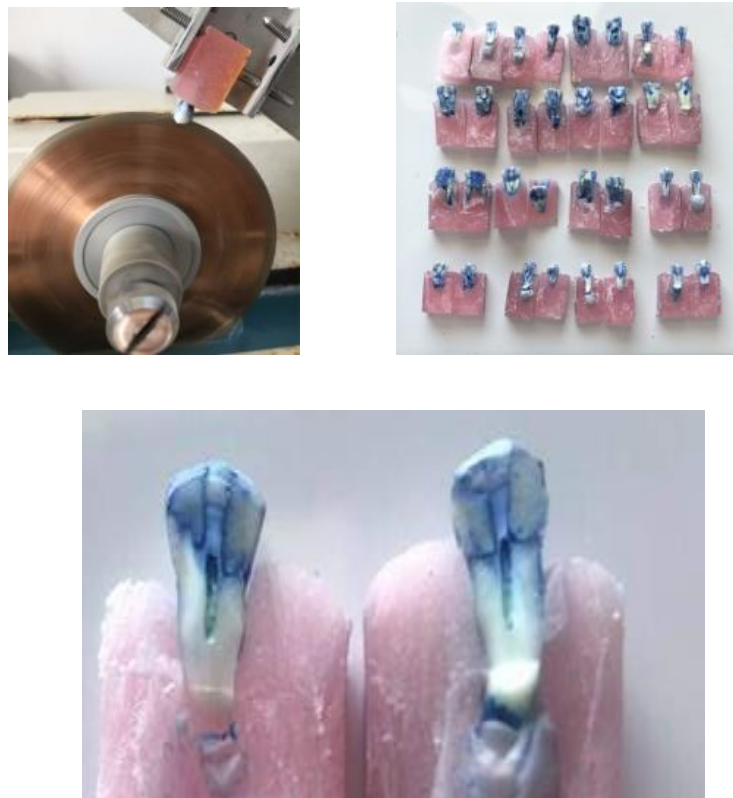
Fig. (5). Cutting teeth with the micrometer (Bueheler IsoMet) in the mesiodistal sense.
